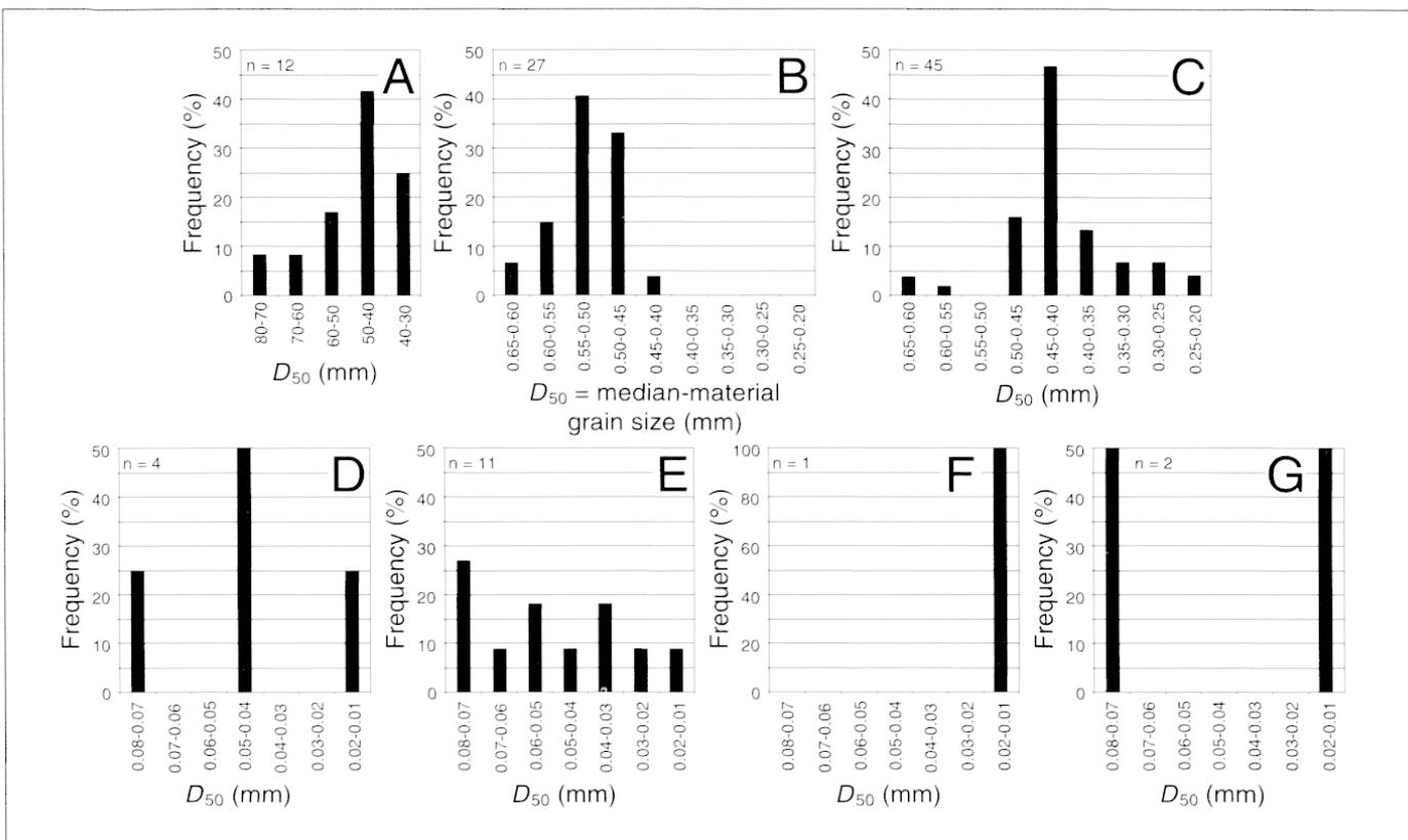
**Fig. 4 – Median grain-size frequencies of bed-material type in the Rhône Delta.** A: cobble-pebble beds of the Grand Rhône; B: sand beds of the Grand Rhône; C: sand beds of the Petit Rhône; D: compact silt beds of the Grand Rhône; E: compact silt beds of the Petit Rhône; F: river mouth mud bed in the Grand Rhône; G: river mouth mud beds in the Petit Rhône.
