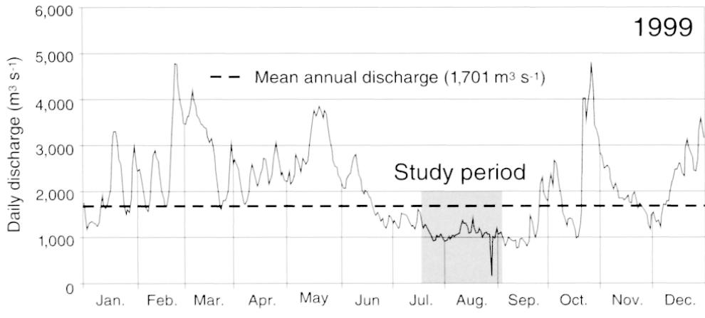
Fig. 3 – Flood hydrograph for the study period. Values are based on gauging measurements at the Beaucaire station (CNR data).
